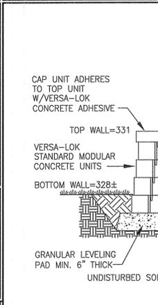
TYPICAL SECTION-UNREINFORCED RETAINING WALL NOT TO SCALE
